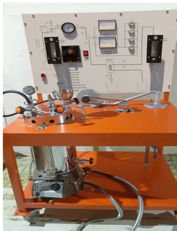
Figure 2. Steam power plant trainer
