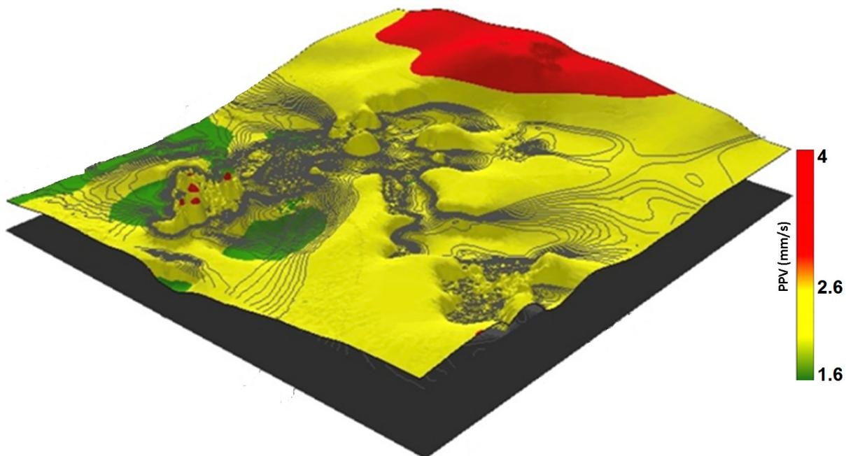
Figure 11. 3-D visualization of spherical Kriging for spatial distribution of PPV in coal mining areas
