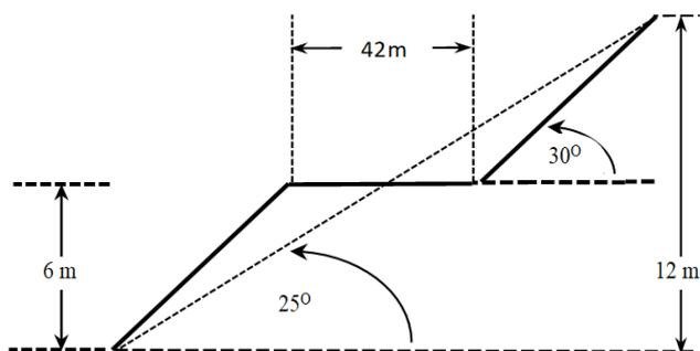
Figure 3. Geometry of drilling and blasting
