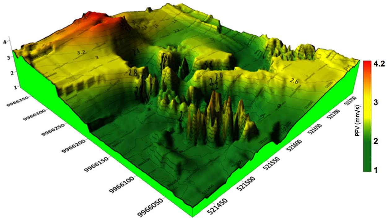
Figure 6. 3-D visualization of the Kriging results of PPV data with mm/s units using the OK method.
