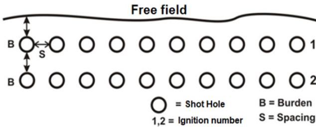
Figure 2. Drilling and blasting patterns
