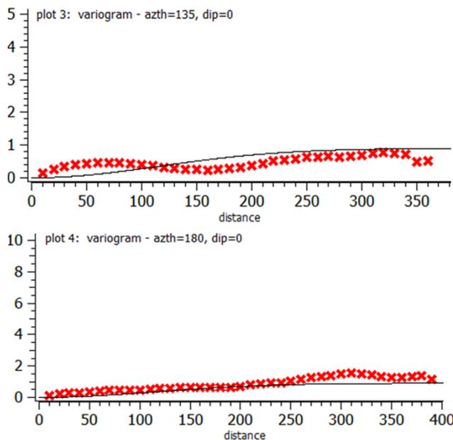
Figure 9. Plot 3 for PPV variogram model, azimuth 135, DIP 0; and Plot 4 for PPV variogram model, azimuth 180, DIP 0
