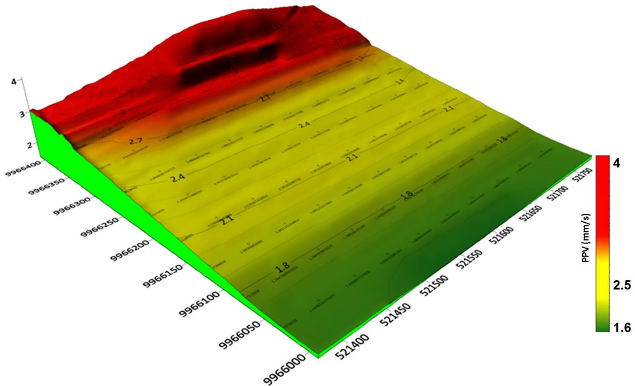
Figure 13. 3-D visualization interpolation results using the spherical Kriging method
