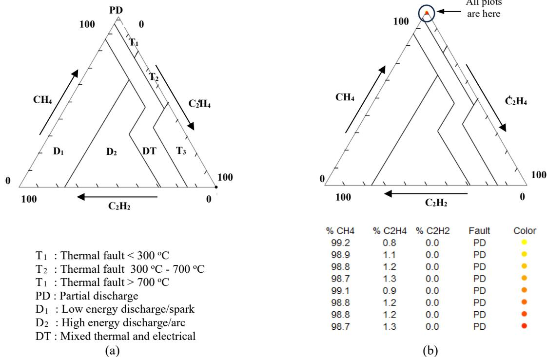
Figure 4. Duval Triangle: (a) each area in the triangle represents a specific fault type, (b) resulted plots of all cases
