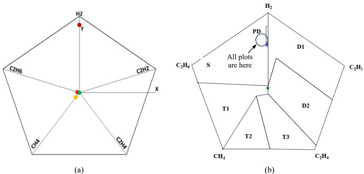
Figure 5. Duval Pentagon; (a) Duval Pentagon 1, dots represent the percentage of each gas in the pure methyl ester under the PD at 20 kV; (b) Duval Pentagon 2, dots represent the resulted centroids of all samples.
