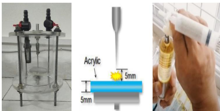
Figure 2. Oil treatment; (a) oil chamber, (b) electrode configuration for PD generation, and (c) syringe for gas-in-oil extraction.
