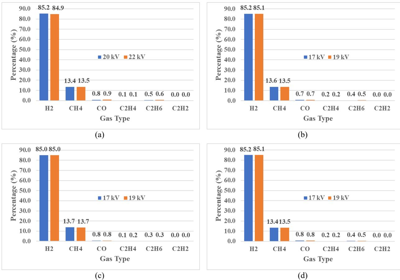
Figure 3. Proportion of a particular gas to the total combustible gases in oil samples: (a) pure methyl ester, (b) ME95-MO05, (c) ME92.5-MO7.5, (d) ME90-MO10
