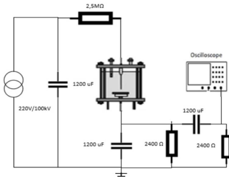
Figure 1. Experimental setup for PD test
