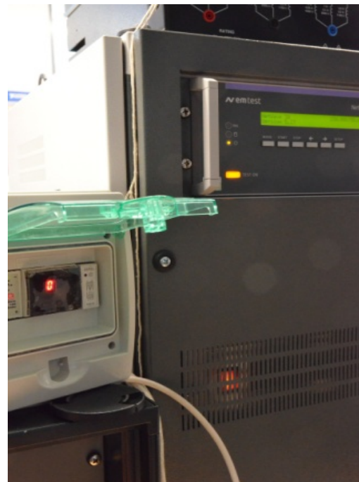
Figure 5. Conducted disturbance measurement
