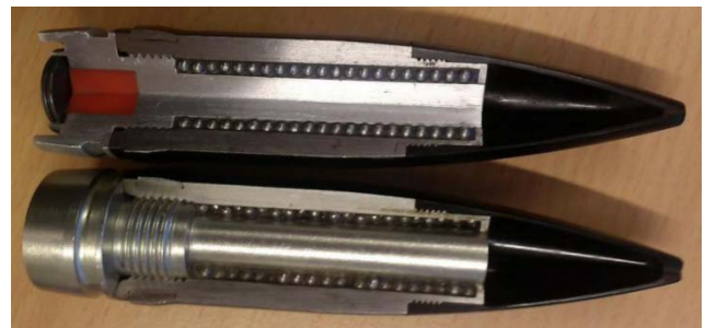
Figure 1. PELE projectile 25x137 mm (casing in lower part filled with spherical fragments) [5]
