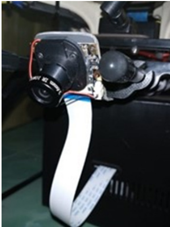
Figure 3. The OV5647 camera module is mounted on the quadcopter
