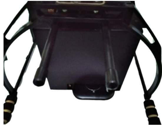
Figure 6. Placement of Wi-Fi module on the quadcopter
