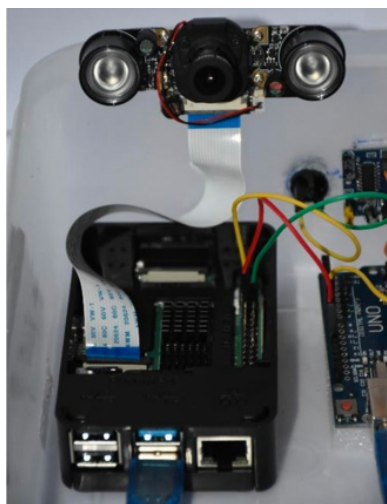
Figure 5. The connectivity between the Raspberry Pi 4 and the camera module
