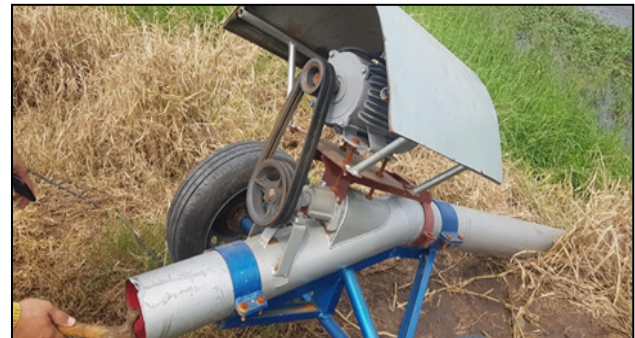
Figure 6. The pipe-type water pump to drain flood
