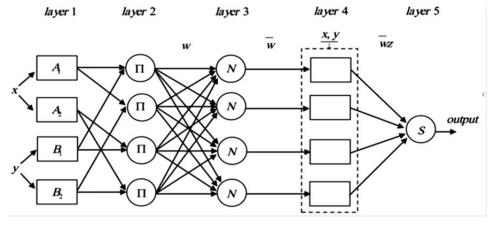
Figure 1. The architecture of the general ANFIS System
