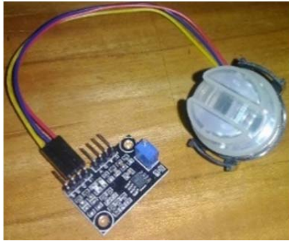
Figure 2. GE turbidity sensor
